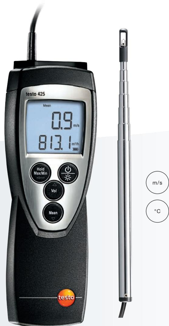
testo 425 is a compact anemometer with a fixed thermal flow velocity probe. The probe head has a diameter of 7.5 mm. With the extendable telescope (length max. 820 mm), the measuring instrument is suitable for flow velocity measurement in ducts. The testo 425 also measures extremely accurately in the low flow velocity range. The volume flow is directly shown in the display. For the purposes of volume flow calculation, the duct area can be
