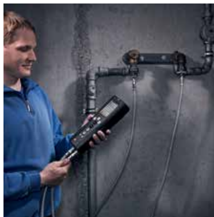
Servicability test without gas-feed appliance
