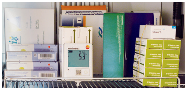
The WiFi data loggers in the drugs refrigerator immediately provide the staff with an alarm when upper or lower limit values are exceeded.
